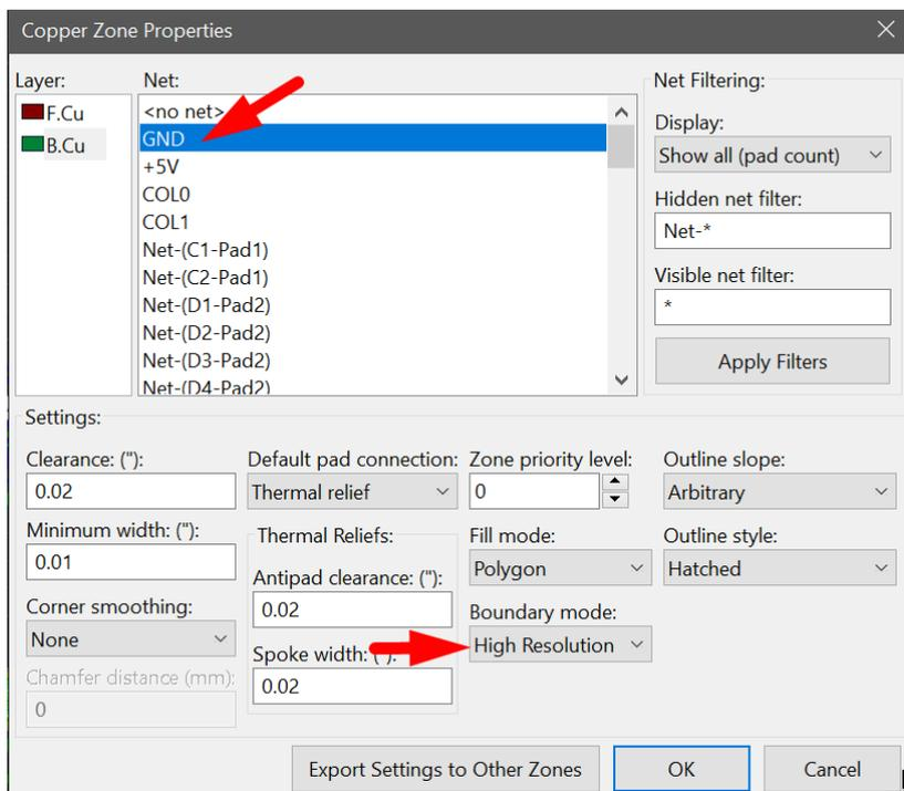
Select the ground net for the fill net, and high resolution for prettier edges.
